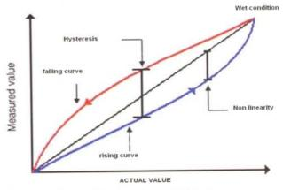
Figure 1. Effect of Hysteresis on moisture measurement.
